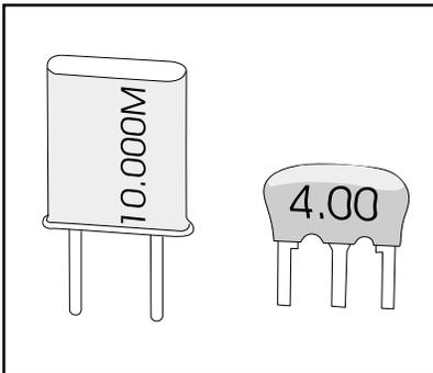
A typical crystal (left) and resonator.
