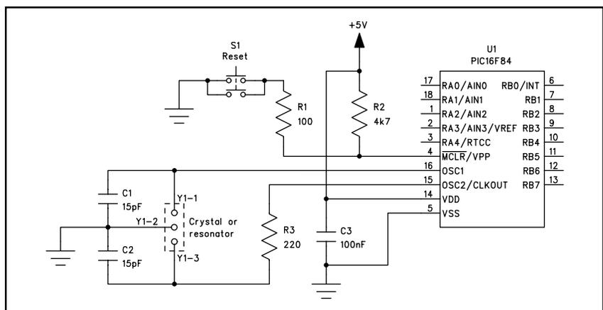
*This schematic diagram illustrates both the clock oscillator and reset circuits.*
